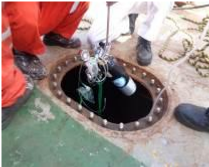
RESUSCITATION EQUIPMENT/FIRST AID KIT LOWERED INTO TANK
